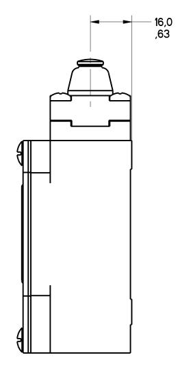
FIGURE 4 - TOP PIN PLUNGER HEAD OTHERWISE REFER TO FIGURE 1
